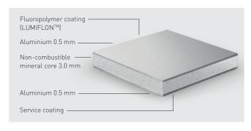
ALPOLIC<sup>TM</sup> A1 is manufactured from two 0.5 mm thick aluminium cover sheets. These are applied to the non-combustible mineral core (3.0 mm) in a special fusing process. The particularly durable fluoropolymer resin coating LUMIFLON™ is applied to one side of the cover sheets in a coil coating process using latest coil coating technology.
