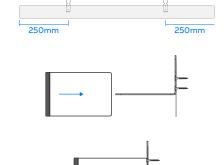
Fix 2 number MP brackets, per linear meter, to the substrate at maximum 250mm from the end of the cavity barrier, with a maximum spacing between brackets of 500mm.
