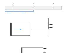
Fix 3 number MP brackets, per linear meter, to the substrate at maximum 150mm from the end of the cavity barrier, with a maximum spacing between brackets of 350mm.
