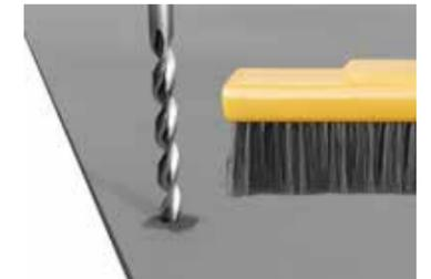
If not using Cembrit Facade Wing Screws, the boards should be pre-drilled with an appropriate fibre cement drill bit. Dust from cutting or drilling must be removed with a brush immediately after the work has been completed, otherwise it can mark the surface of the boards.
