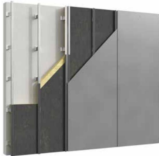
Wall with brackets, vertical steel Omega and U profiles
