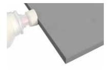
All cut edges (except Cembrit Patina design line boards) must be sealed with Cembrit Edge Sealer to ensure protection of the cut edges. Use the Cembrit Edge Sealer Set with Applicator and Sponge. Avoid getting Edge Sealer liquid on board faces. If this does occur, remove any liquid with a lint-free cloth immediately.
