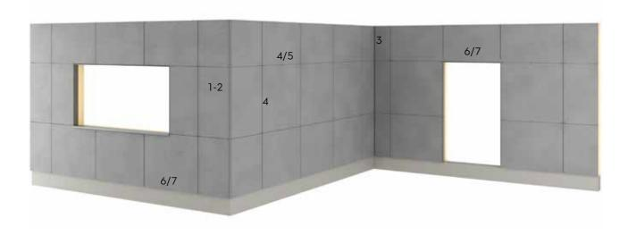
One way to create an aesthetically pleasing solution, is to use the Cembrit corner profiles as shown here. As the other profiles, the corners profiles are available in a variety of colours to match your facade boards.
