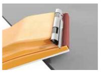
Once boards are cut, you can bevel the cut edge with a fine grinder (80 grain) to give the edge a pre-cut finish.
