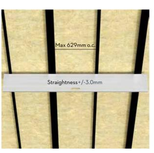
Straightness of substructure
