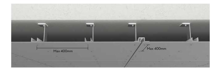
When using Cembrit facade boards as ceiling or soffit, you can normally use a regular steel system with steel profiles, but for larger cavities, you need to contact an steel manufacturer to make sure the system fits your needs. The number of brackets and types of anchoring used for the type of deck/ceiling has to be calculated, and the manufacturer's instructions should always be followed.
