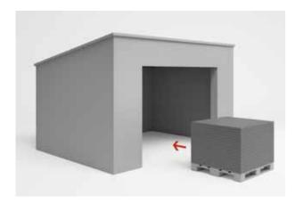
If Cembrit facade boards are stored more than 2-3 weeks on site, the pallets should be kept under a roof to ensure dry and ventilated conditions.
