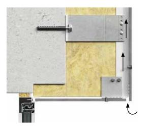
A horizontal free ventilation opening must be maintained above windows and doors as well. This ventilation gap must be at least 10mm wide. If steel, aluminium or plastic perforated profiles are used, a ventilation area opening of minimum 100cm<sup>2</sup> per meter
