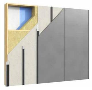
Light wall with vertical VFL steel profiles
