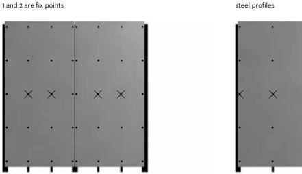
Example: Vertically mounted boards with one intermediate steel profile
