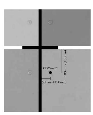
Example of vertical substructure
