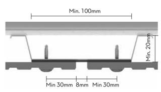
Fig. 1. Cembrit Patina Inline installation on profile behind joint.
