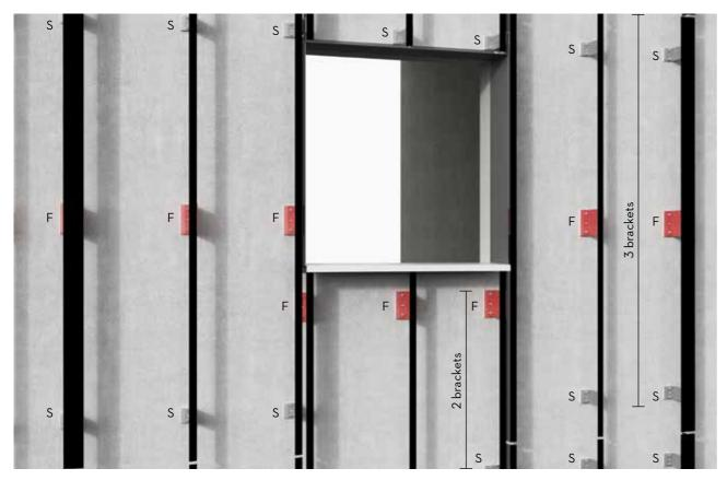
Red brackets are the brackets with fixing points (F)
